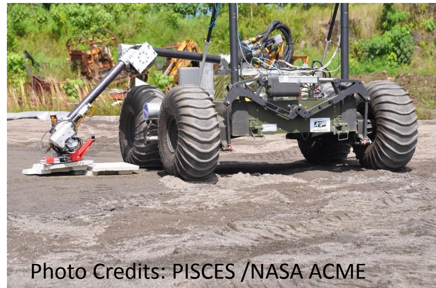
NASA/ PISCES Paver Laying Robot
