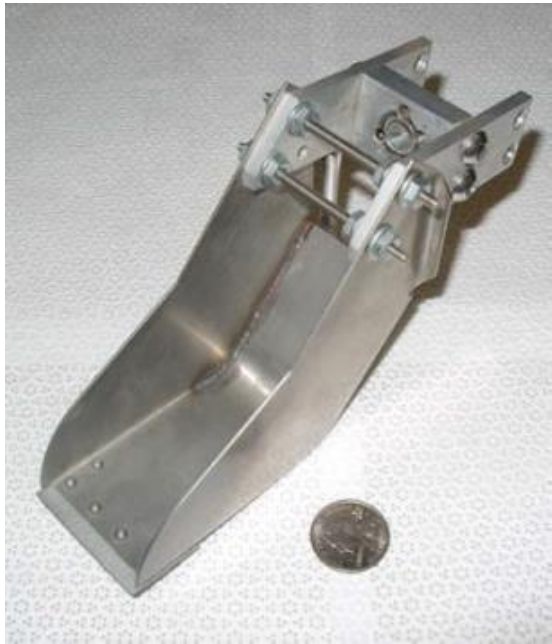
Replica of NASA Lunar Surveyor Scoop & Test results in regolith simulants
