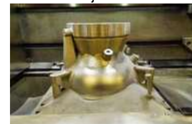
28-element Inconel 625 fuel injector
