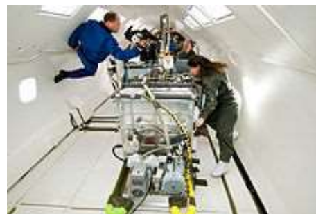
EBF 3 wire-fed system during parabolic flight testing
