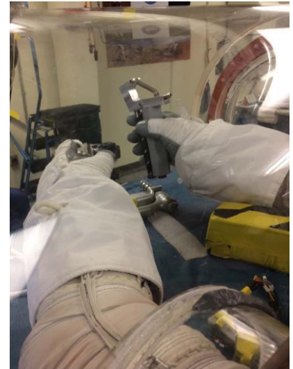
Figure 2. Experimental setup showing a subject wearing the SSRG and squeezing a dynamic gripper inside of the glove box.
