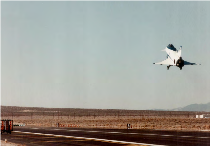
The X-31 executing a go-around following its simulated carrier approach; note the FLOLS in the lower left of the photograph. (NASA DFRC)
