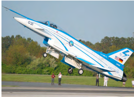
X-31 VECTOR landing just prior to derotation. Note the nozzle paddles far below the main landing gear. (USN)
