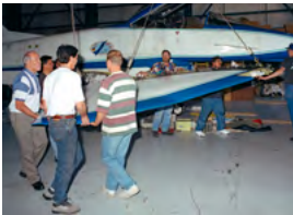
Left to right: Dance of the Disassemblers: removing the right wing so that the X-31 could fit into a Lockheed C-5 for airlift to Europe. The X-31 being loaded into an Air Force Reserve C-5. All tucked away, nice and snug. (NASA DFRC)
