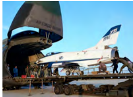
Left to right: Dance of the Disassemblers: removing the right wing so that the X-31 could fit into a Lockheed C-5 for airlift to Europe. The X-31 being loaded into an Air Force Reserve C-5. All tucked away, nice and snug. (NASA DFRC)
