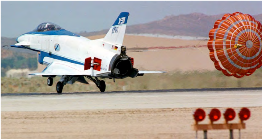
Drag-chute testing at Edwards in preparation for Paris. (NASA DFRC)
