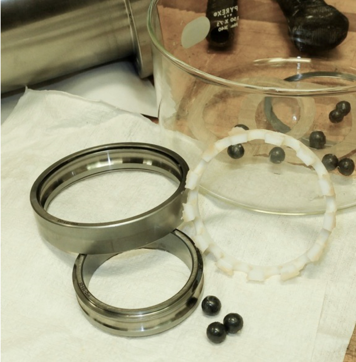
Figure 14.—Photograph of high quality 60NiTi ball bearing during post-test (5000-hr) inspection in which no grease degradation, wear or fatigue was observed.
