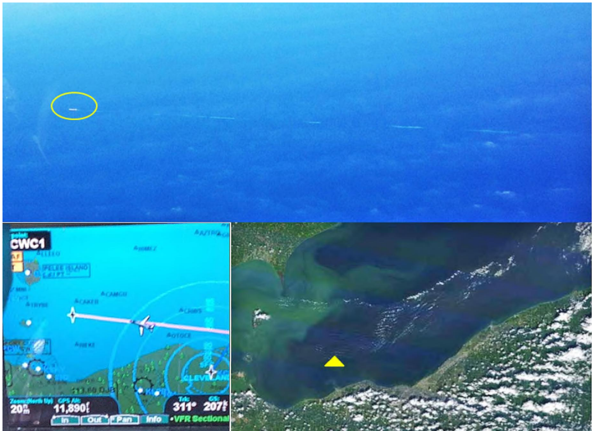
Figure B.3.—Contrasting airborne image with MODIS (Moderate Resolution Imaging Spectroradiometer) satellite image (lower right).
