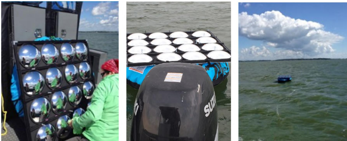
Figure 3.12.—Pictures of the 16 mirror array (left), it floating in the water near the boat (center), and the floating mirror target as deployed away from the boat during overflight.
