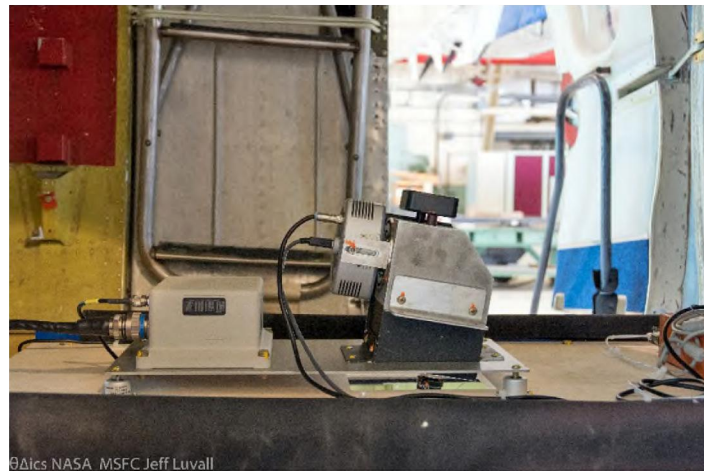
Figure 1.3.—Imager and inertial navigation system mounted in Twin Otter aircraft.
