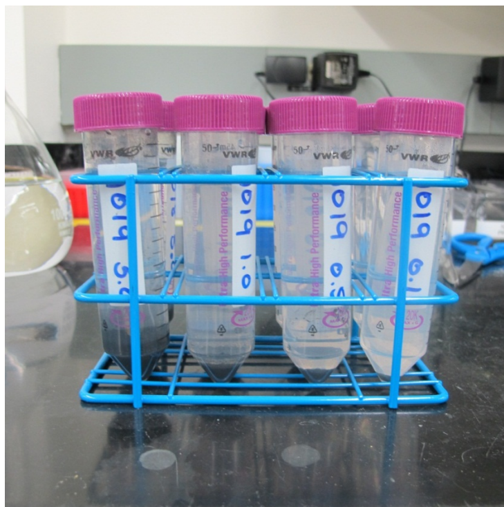
Figure 16. Plastic Test Tubes with Varying Amounts of Organic Adsorbent and Glutaraldehyde Test Solution
