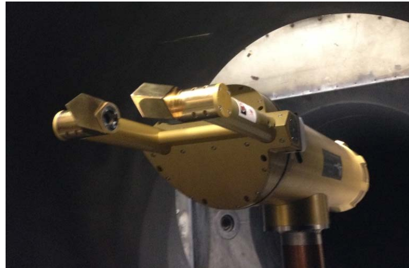
Cloud Imaging Probe (CIP-GS) Shadowing
