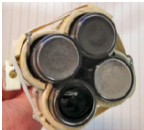
Figure 2.—End-on view of four test specimens in vials prior to LINAC beam exposure. Center of holding fixture aligned with beam centerline. Vial-to-vial (diagonal) distance nominally 2.5 cm (1 in.).
