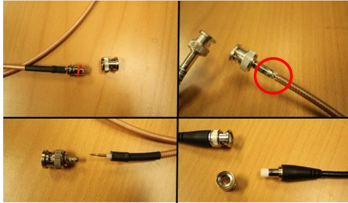
Figure 9. Antenna Cable Connector Failures from Strength Testing
