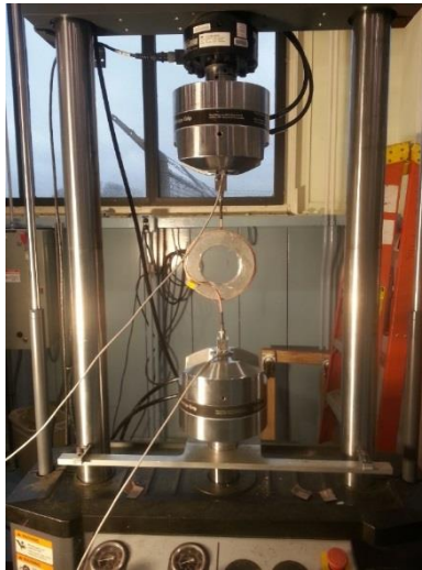
Figure 8. Antenna Cable Tensile Test Setup
