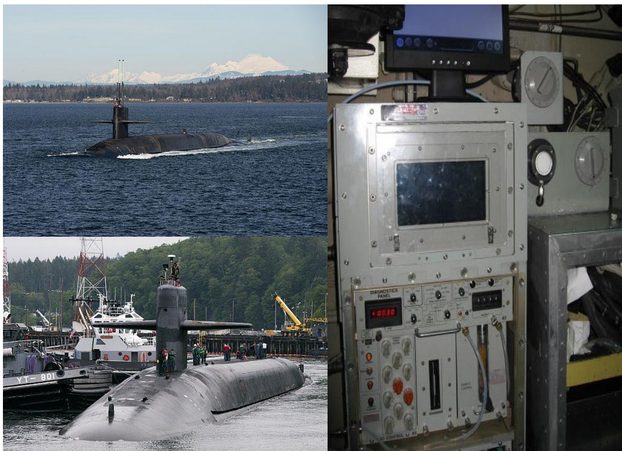
Figure 3. Nuclear powered Ballistic Missile Submarines the USS Henry M. Jackson (upper left) and the USS Alaska (lower left) with a typical Central Atmosphere Monitoring System (CAMS Mk II) rack mounted in the fan room. This is a potential location for MGM during the sea trial. Photo source: www.navy.mil
