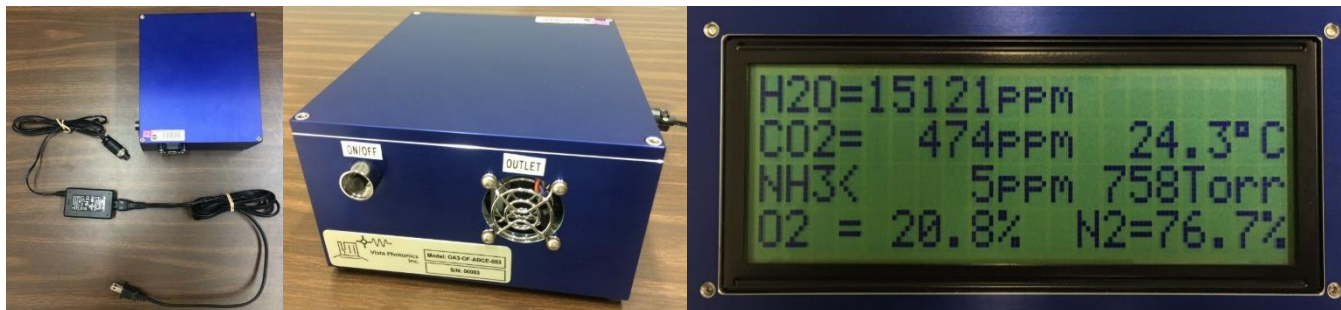
Figure 2. Sea trial MGM with power cord/adaptor (left). A single button powers it ON/OFF (center). A small 5V fan pulls in air sample into the interior cell where the measurements occur and exhausts at outlet. The display (right) reflects the concentrations, temperature, pressure and Nitrogen (N 2 ) by difference, assuming cabin atmospheric Argon at 0.9%.
