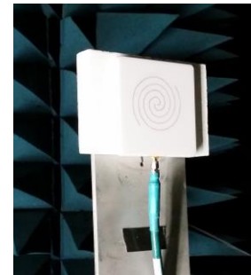
3-D Printed Antennas for Cubesats
