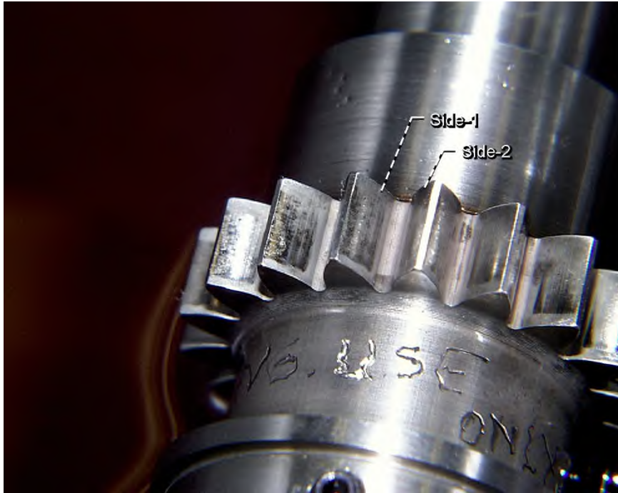
Figure 3.20.—Driven side of pinion gear teeth after the test Final-5 are still in good condition.
