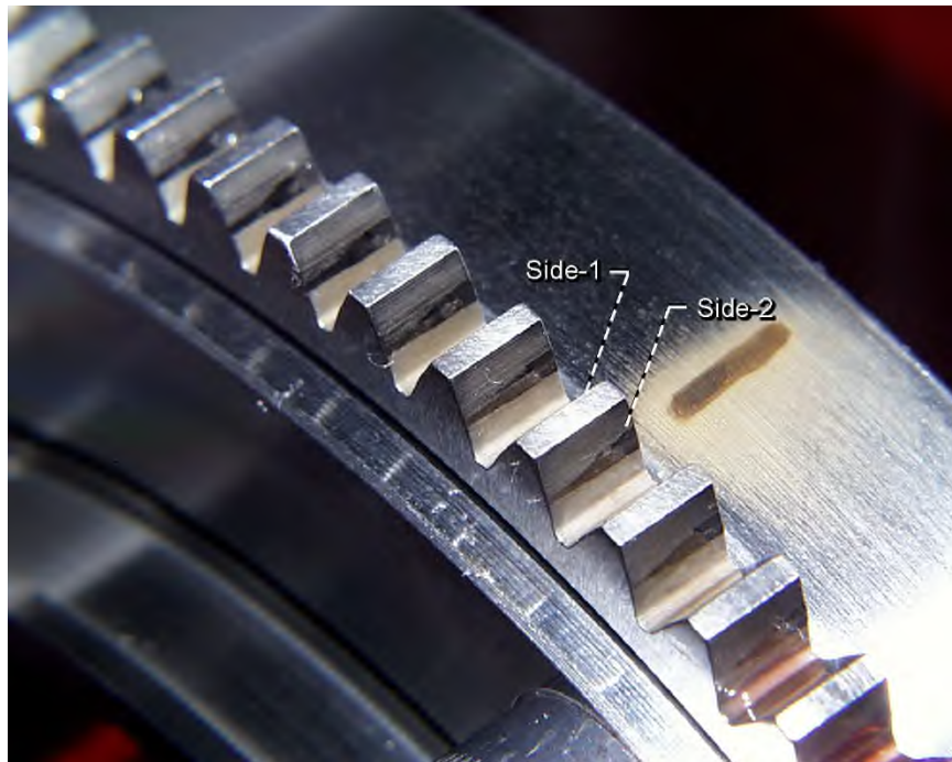
Figure 3.16.—No visible damage on driving side of ring gear teeth after Score-1 test on side-2, build-1.
