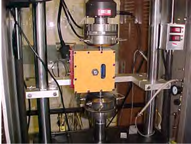
Figure 2.3.—Test fixture in tensile test machine.
