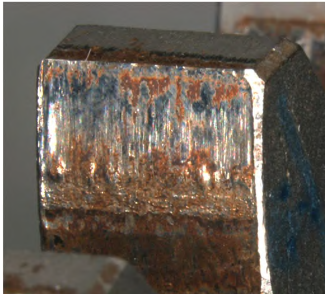
Figure 4.6.—Typical condition of the worn gear teeth.
