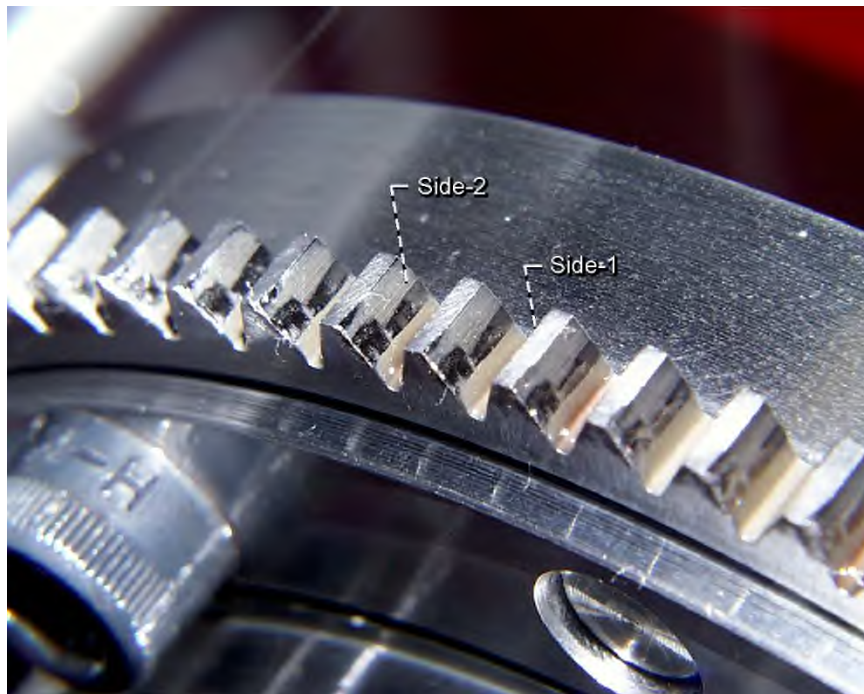
Figure 3.19.—Damaged teeth of ring gear after disengagement at 14,000 rpm pinion speed during the score-2 test on side-2, build-1. White cloth fibers are caught on teeth from wiping oil.
