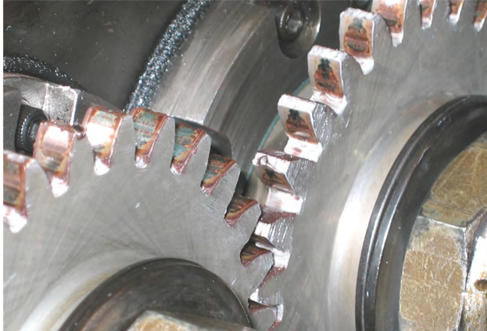
Figure 1.2.—Condition of the test gears after 3 hr of operation for test number 1 having test conditions of perfluoro type grease, 515 rpm shaft speed, 5 ft-lb torque, and ambient air atmosphere.
