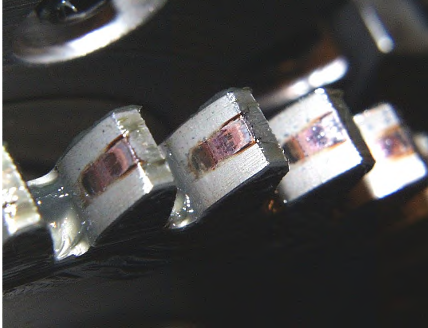
Figure 1.10.—Condition of the driven gear after 1 hr of testing for test number 6 having test conditions of hydrocarbon-based grade 2 grease, 214 rpm shaft speed, 2 ft-lb torque, and ambient air atmosphere.
