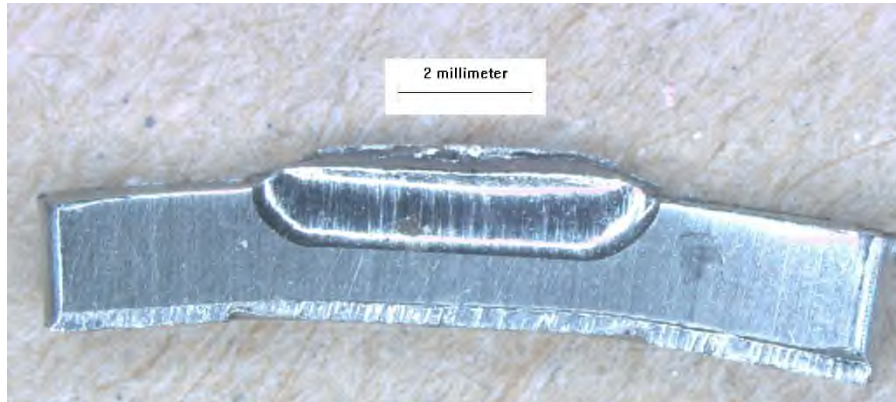
Figure 6.5.—Example of deformed shim stock after engagement of meshing gear teeth.
