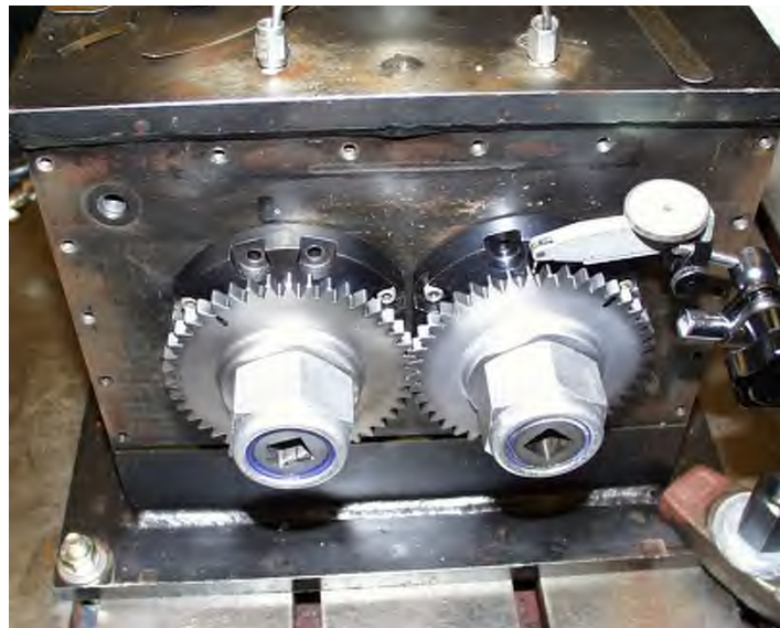
Figure 6.2.—Setup for backlash measurement using dial indicator.
