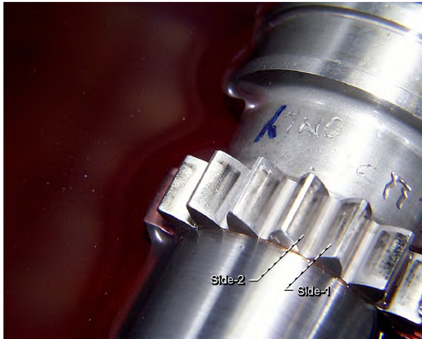
Figure 3.15.—Wear marks on driven side of pinion gear teeth after Score-1 test on side-2, build-1.
