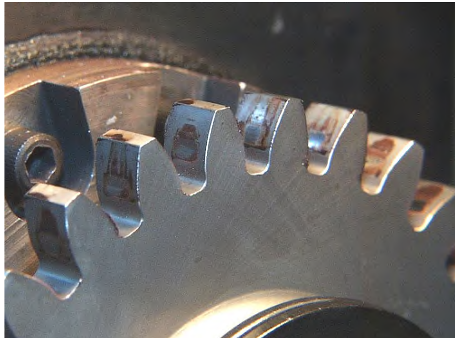
Figure 1.11.—Condition of the driven gear after 1 hr of testing for test number 7 having test conditions of no lubricant, 705 rpm shaft speed, 2 ft-lb torque, and ambient air atmosphere.
