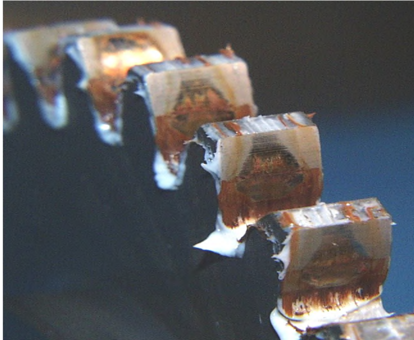
Figure 1.6.—Condition of the driven gear after 15 hr of testing for test number 2 having test conditions of perfluoro type grease, 200 rpm shaft speed, 2 ft-lb torque, and ambient air atmosphere. A mixture of original white and red colored grease is evident along with wear patterns.
