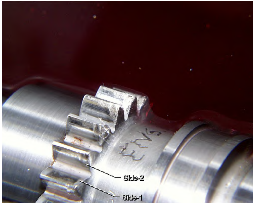
Figure 3.18.—Damaged teeth of pinion gear after disengagement at 14,000 rpm pinion speed during the Score-2 test on side-2, build-1. White cloth fibers are caught on teeth from wiping oil.
