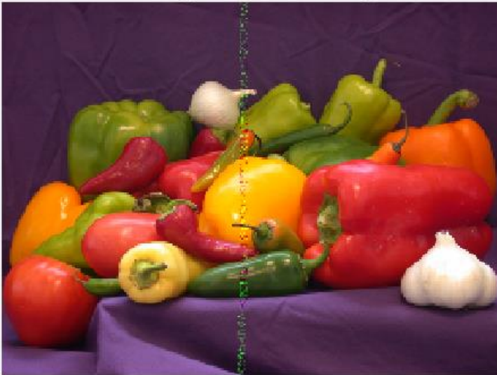
Figure 8. Image transmitted at 62 dB after 50 krad(Si) for DUT3.
