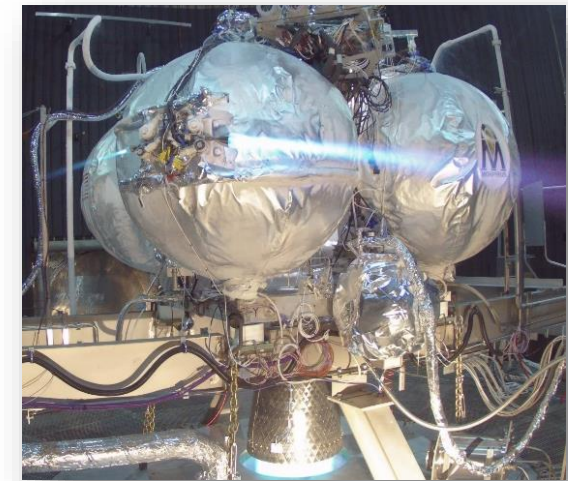
ICPTA Simultaneous Hotfire at NASA Plum Brook B2, 2/28/17
