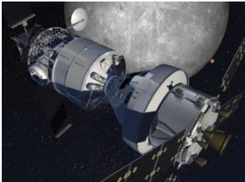
Figure 34. Concept of typical NASA Crew Transit Stage (CTS) with COV docked. (Credit: NASA)
