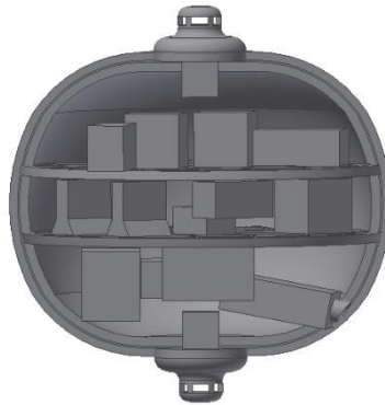
Figure 34 Section cut of the Payload Module
