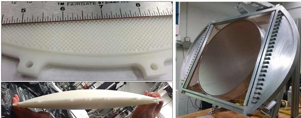
Figure 9. Left Figure: (Bottom) The 40 cm diameter 1 Kelvin high density polyethylene lens for the 38 GHz telescope. (Top) A close up of the simulated dielectric anti-reflection coating used for all plastic cryogenic optics in the 38 GHz telescope. Right Figure: The variable-delay polarization modulator (VPM) for the CLASS 38 GHz telescope. The wire grid contains over 3000 50\mu\text{m} copper plated tungsten wires spaced 150\mu\text{m} apart across a 61 cm clear aperture. A 60 cm flat aluminum honeycomb mirror attached to a mirror transport mechanism sits behind the wire grid and creates a phase delay between polarization states parallel and perpendicular to the wire grid which is modulated at 10 Hz.
