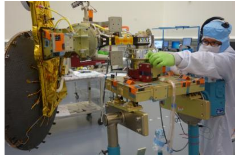
Antenna Assembly – range of motion testing
