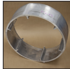
Aluminum Cylinder with 1 Inch Tall Stiffeners (17 in. dia.)
