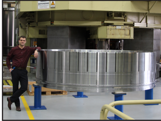
Slotted mandrel for forming 10-foot diameter integrally stiffened cylinder in 2017.
