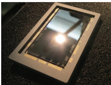
2-D-doped EMCCD with custom AR coating for FIREBALL and Palomar observations. (Credit: Todd Jones)
