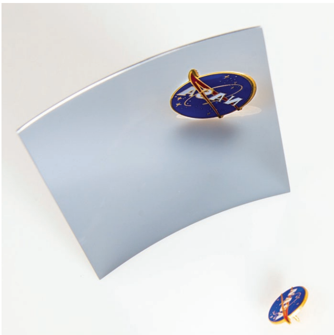
A Wolter-I mirror segment with a thickness of 0.6 mm. This mirror has a dimension of approximately 100 mm by 100 mm. Tens of thousands of mirror segments like this one will be aligned and integrated to make an assembly to achieve several m^2 of effective area. (Credit: Bill Hrybyk)
