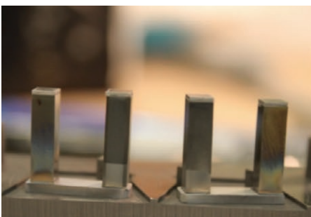
Left: New industry-produced SKD couples that are resilient enough to operate in the eMMRTG hermetically sealed converter cavity. (Credit: S. Keyser, Teledyne Energy Systems, Inc.) Center: Monte Carlo simulation of heat flow across composite TE material with metal inclusions. (Credit: P. von Allmen, JPL/Caltech) Right: High-temperature segmented thermoelectric module technology with 2X efficiency gain over heritage RPS technology. (Credit: S. Firdosy, JPL/Caltech)
