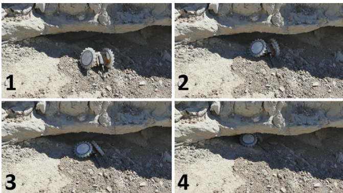
PUFFER prototype collapsing to drive beneath a natural overhang during field testing in the Mojave Desert.
