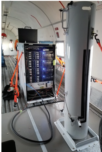
UWBRAD instrument installed in the DC-3T aircraft. The cylinder in the foreground is the deployable "periscope" antenna, and the instrument electronics are housed in the rack in the background. (Credit: Joel Johnson/OSU)
