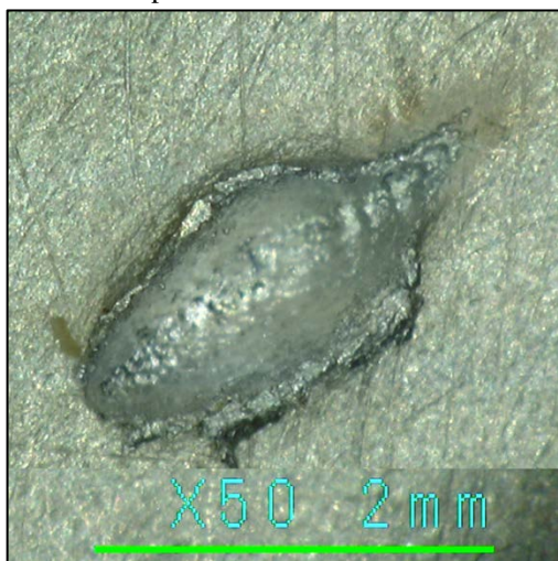
Figure 13. 2.4 x 0.9 mm impact crater on airlock panel
