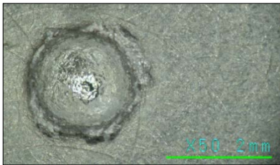
Figure 17. 1.8mm diameter crater in airlock (33-1)
