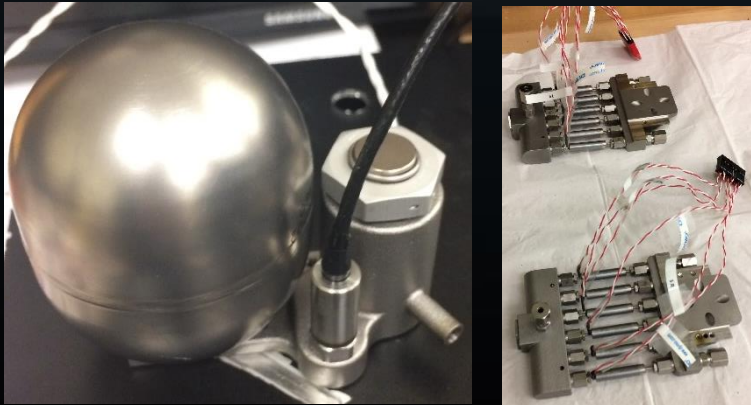
(L) Tank, iso valve and transducer mounted on 3-D printed tank boss and (R) Thruster valves assembled with 3-D Printed thruster clusters
