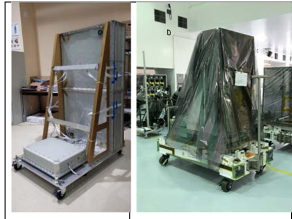
Figure 6. Left: The SDS flight unit. The sensing surface is to the right. The dimensions are approximately 172 cm (height) x 122 cm (width). Right: SDS in the Intermediate Bay at NASA/KSC ready for launch.
