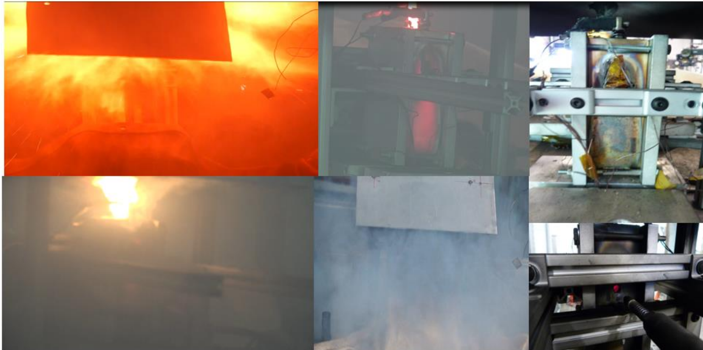
Trigger Method testing on Quallion Cells – Left two are of cell in TR, Middle two are cell venting, Right two are post test pics
