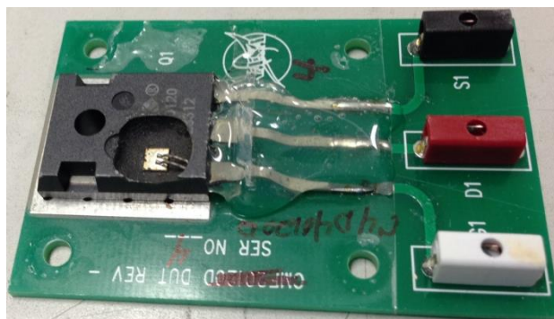
Figure 1. Pin-out of C4D40120D (left) and photograph of decapsulated TO-247 packaged DUT mounted on a daughter card (right).
