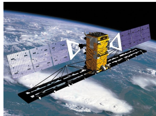
Fig. 2. Canadian RadarSat2 with two symmetric solar arrays (deployed sideways) and one large deployed radar array antenna (downward facing), (image credit: CSA)
