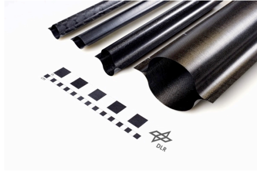
Fig. 9: DLR composite booms of different scale [Source: DLR]
