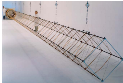
Fig. 12: Deployed FAST mast as used on ISS (Courtesy of Able Engineering – Extracted from [7])
