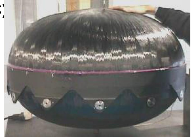
DAWN Tank prior to installation of MLI and external heaters. [ref1]
