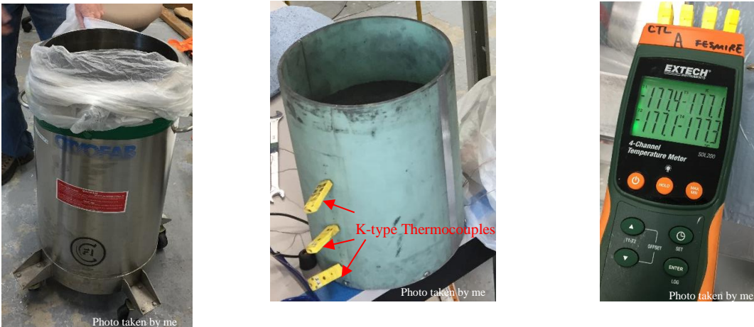
Figure 6. Left: The Cryofab used for the thermal cycling experiment Middle: The sample holder with the K-type thermocouples Right: Temperature meter showing temperatures for the thermocouples
