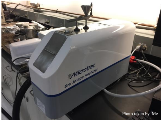
Figure 1. Microtrac PartAn Mini used to analyze Orgueil simulant
