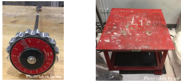
Figure 4. Left: Picture of Humboldt geovane shear soil strength tester Right: Picture of vibrating table used to compact samples
