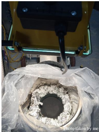
Figure 8. The second set-up for the thermal cycling experiment where we placed aluminum foil around the sample holder preventing light from shining on the bottom
