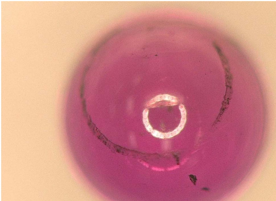
Figure 19 - Sapphire Ball from 1st Stage Regulator
