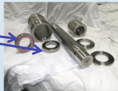
DA Centrifuge Bearing Test Rig Spindle Components
