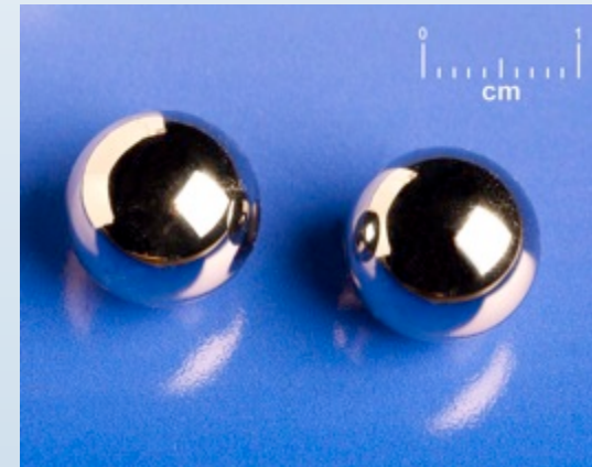
Highly polished 60NiTi bearing balls
