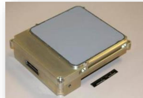
Prototype Tile PAA in Airborne Packaging
