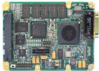
Proton 400k Rad-Hard Processor
