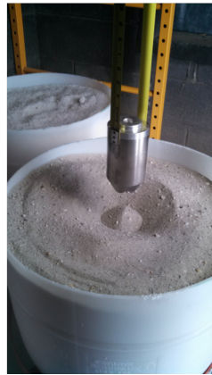
Figure 17. Barrel of Comet Material Simulant Installed in TTF Showing Dual Carpenter's Tape Tether and SARP Having Penetrated and Then Extracted from Simulant
