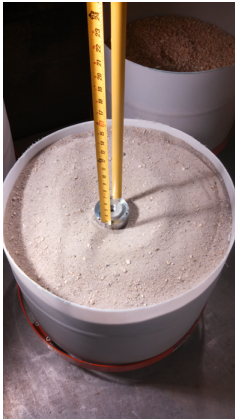
Figure 17. Barrel of Comet Material Simulant Installed in TTF Showing Dual Carpenter's Tape Tether and SARP Having Penetrated and Then Extracted from Simulant
