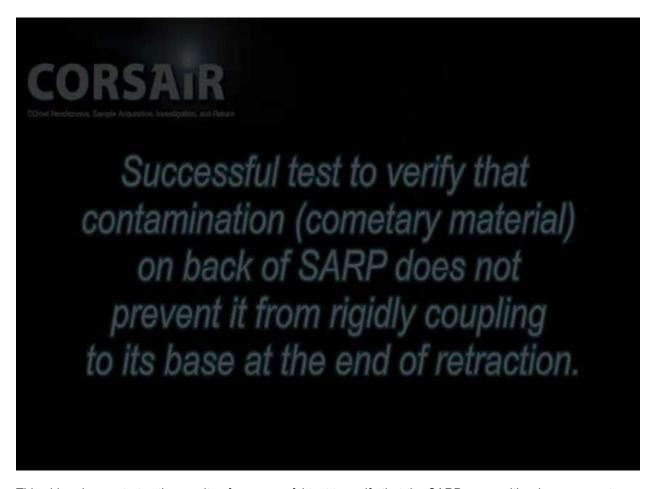
This video demonstrates the results of a successful test to verify that the SARP, even with a large amount of cometary material adhering to its back side, could still achieve a sufficiently rigid coupling with the interface plate at the end of the birdcage piston, which serves as the mechanical ground for the SARP at the end of its retrieval.
