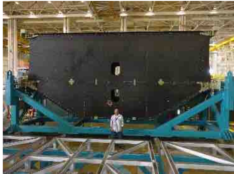
Assembled Multi bay Box in C-17 Factory
