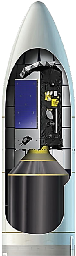
Alphasat in Ariane 5 fairing. (Photo: ESA)
