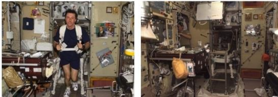
ISS Service Module configuration with galley, treadmill, crew quarters, and waste and hygiene facilities co-located. (from HRP Evidence Report)
