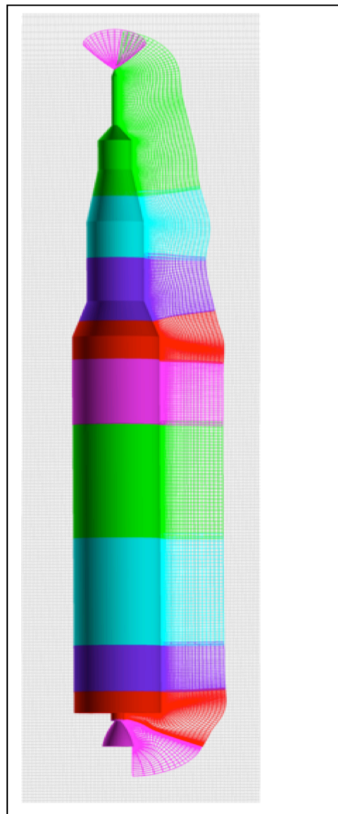
Fig. 2a Portions of near body grids (colored) embedded in off-body grid (grey).
