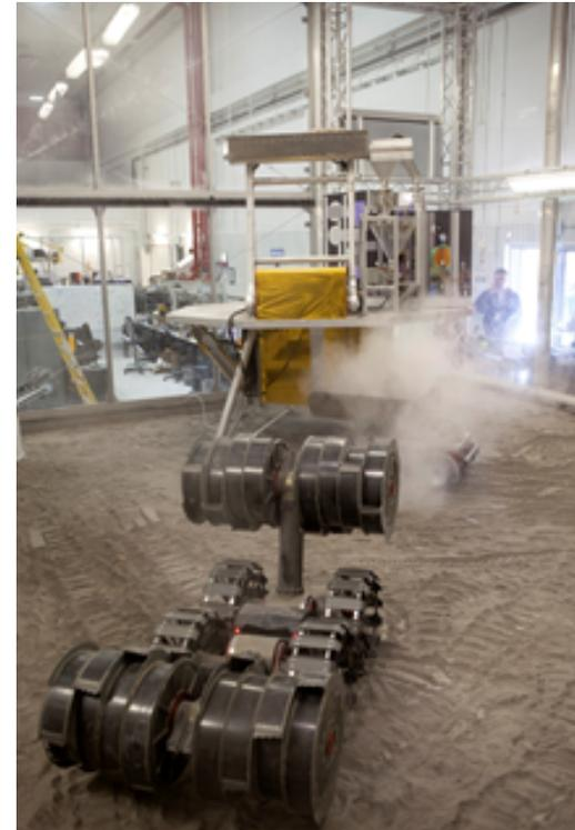
KSC RASSOR (Regolith Advanced Surface Systems Operations Robot) excavator delivering loose soils
