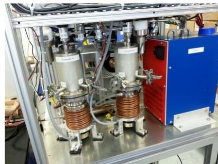
CO<sub>2</sub> freezers and chiller (left) and 3D model (below)
