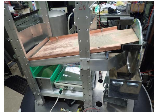
Concept for open water extraction soil processor
