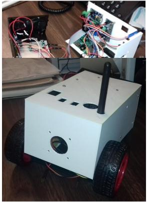
The shell of the robot itself is a 3D printed case that will (work in progress) snap together. The photo to the left shows the two halves separated from each other. The black shell contains the power distribution boards and connectors while the white shell contains the driving base and data systems.
