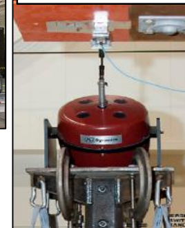
3-DOF Transducer on 100-lbs Shaker
