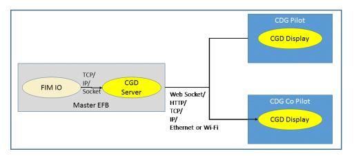
Figure 5 - CGD Software Architecture
