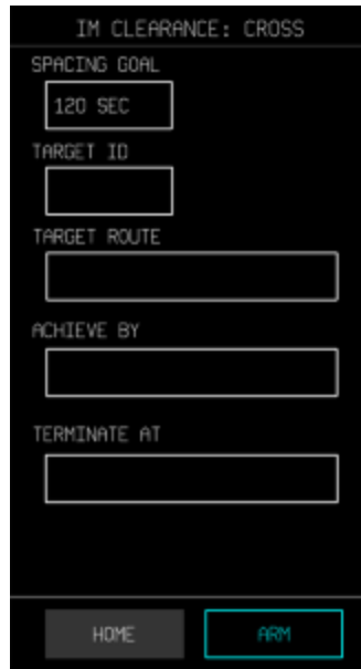
Figure 53. IM CLEARANCE HOME with SPACING GOAL entry made
