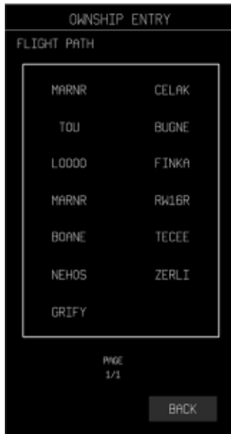
Figure 25. Example of VIEW AS WAYPOINTS selection for the flight path
