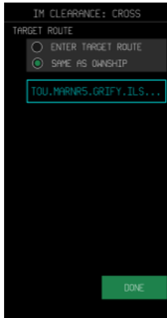
Figure 58. Selection of SAME AS OWNERSHIP for TARGET ROUTE, with DONE button available
