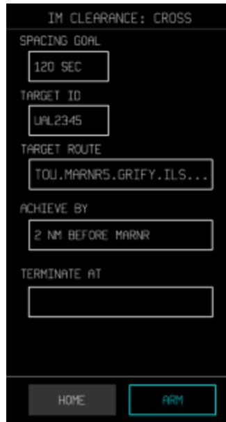
Figure 67. IM CLEARANCE: CROSS home page with ACHIEVE BY field completed
