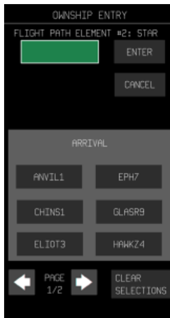
Figure 21. Example list of arrivals for the STAR flight path element
