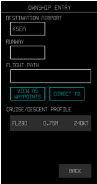
Figure 16. Ownship Entry page after entry of an acceptable identifier for the Destination Airport
