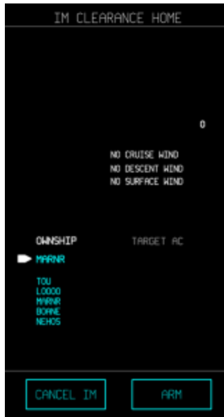
Figure 30. IM CLEARANCE HOME page with the next six waypoints listed under OWNSHIP
