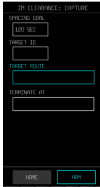
Figure 39. IM CLEARANCE HOME with SPACING GOAL entry made
