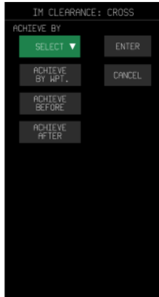
Figure 61. ACHIEVE BY sub-page and drop-down menu after selecting the ACHIEVE BY field
