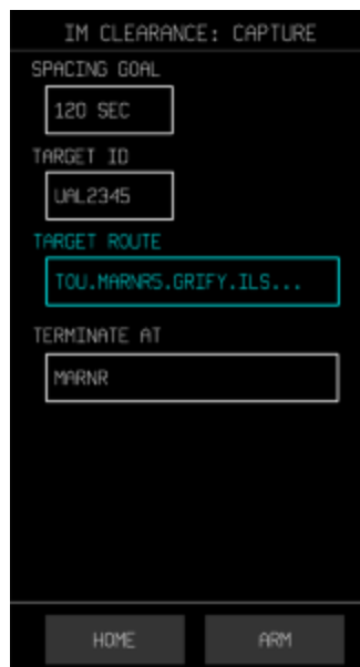
Figure 47. TERMINATE AT field with waypoint entered, and availability of the ARM button
