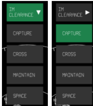
Figure 6. HMI drop-down functionality, including default and active states
