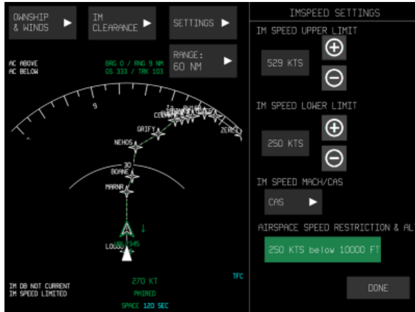
Figure 91. Selection of airspace speed restriction setting
