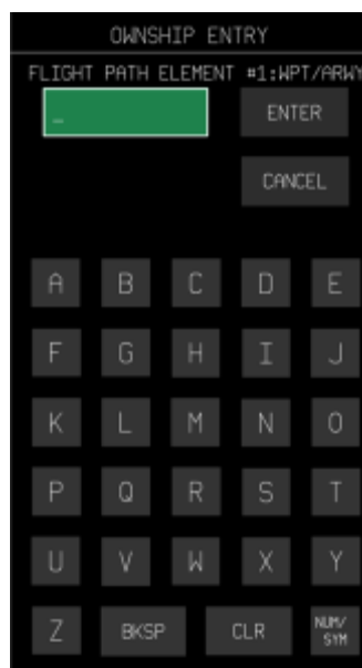
Figure 19. Keypad appearing on selection of WAYPOINT/AIRWAY flight path element type
