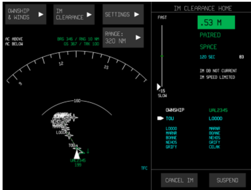
Figure 88. IM commanded speed in “reverse video” at top right
