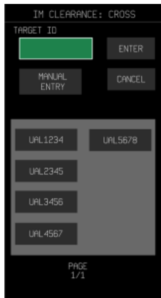
Figure 54. TARGET ID entry page, which appears on selection of TARGET ID field
