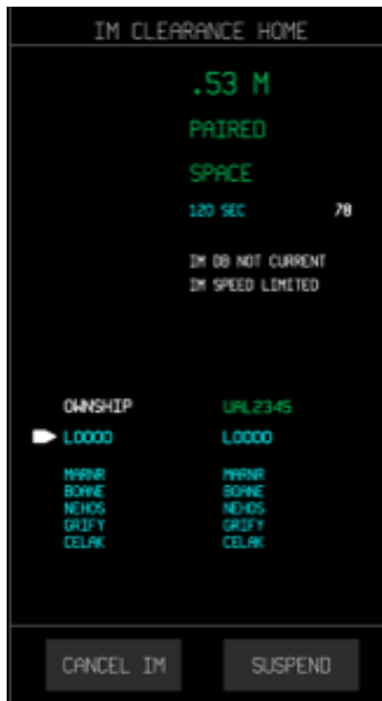
Figure 87. Speed command during the PAIRED state
