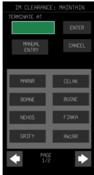
Figure 76. Sub-page that appears after selection of TERMINATE AT WPT
