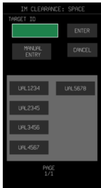
Figure 82. TARGET ID entry page, which appears on selection of TARGET ID field
