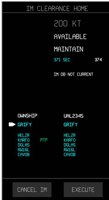
Figure 86. Pending speed command during the AVAILABLE state
