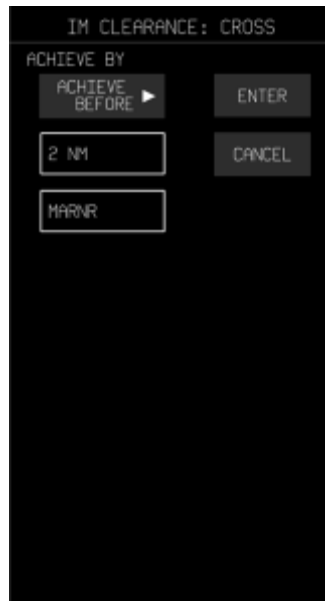
Figure 66. ACHIEVE BEFORE sub-page with entries completed
