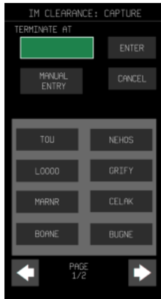
Figure 46. List of selectable waypoints for TERMINATE AT WPT
