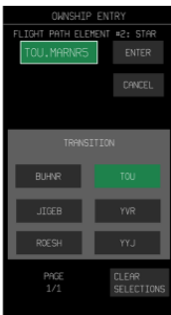
Figure 22. List of Transitions related to a selected STAR flight path element
