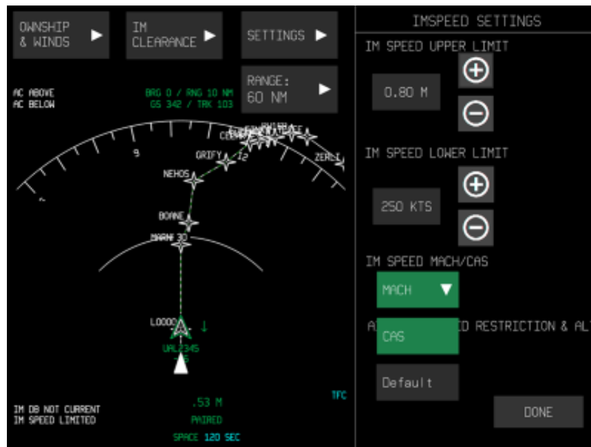
Figure 90. IM SPEED unit selection
