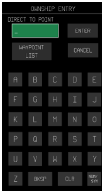
Figure 27. Manual entry of DIRECT TO waypoint
