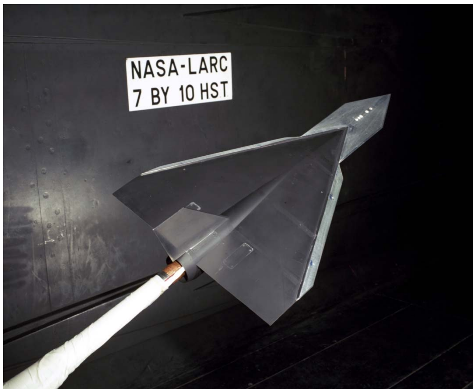
Figure 1. Photographs of the 65° cropped delta wing model installed in the NASA Langley 7- by 10-Foot High Speed Tunnel. (Porous LEX and leading-edge flaps are unpainted surfaces.)
