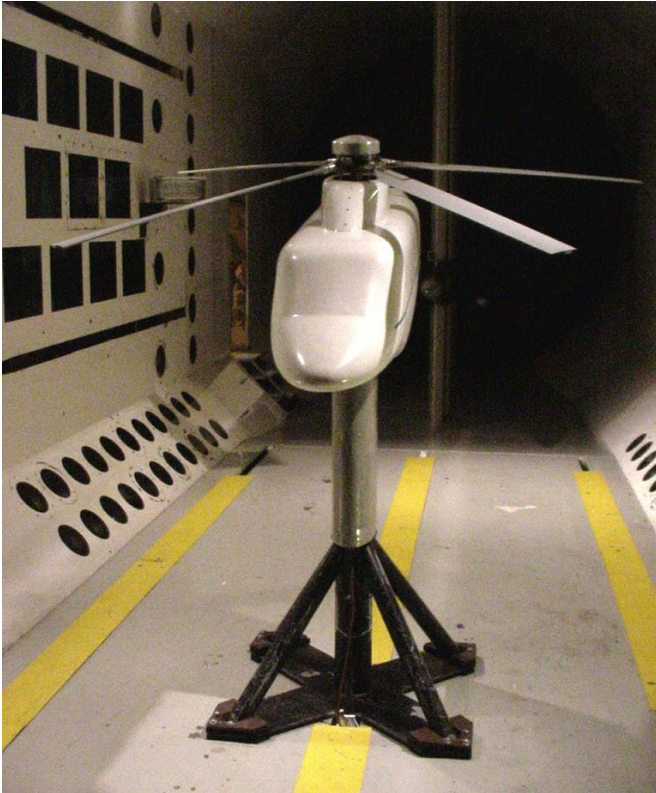
Figure 2. The Aeroelastic Rotor Experimental System (ARES) model-scale helicopter rotor research testbed shown mounted in the test section of the Langley Transonic Dynamics Tunnel (TDT).
