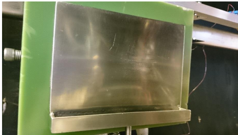
Figure 1. Scavenger Plate in Thermal Vacuum Chamber
