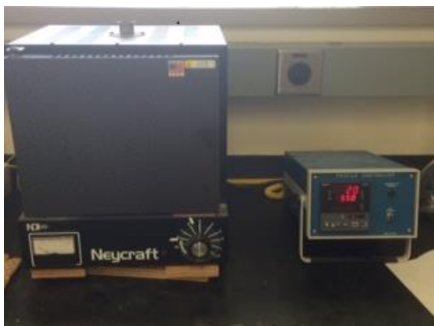
Figure 7. Bake-out Furnace Setup (Building 1293C room 266).
