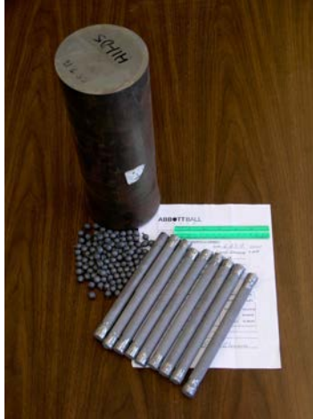
Figure 4. 60NiTi ingots and blanks produced by PM process.
