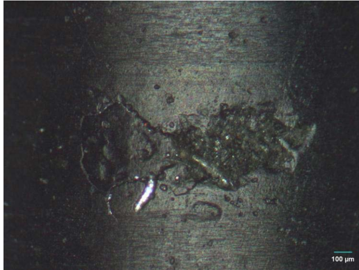
Figure 1. Spall damage on a hardened 60NiTi rod surface following testing at 3.0GPa.
