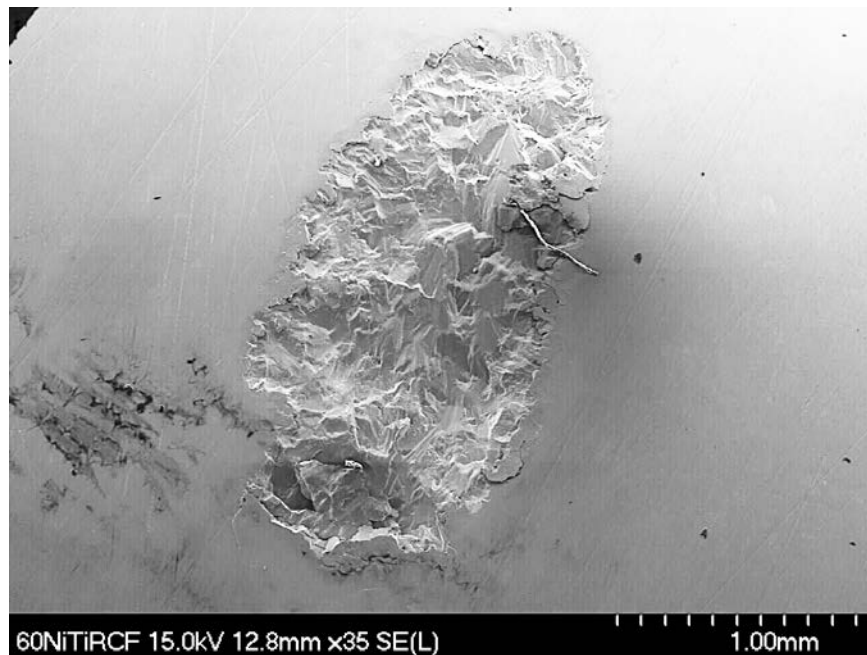
Figure 9. PM-60NiTi RCF rod surface view (SEM) of fatigue spall.
