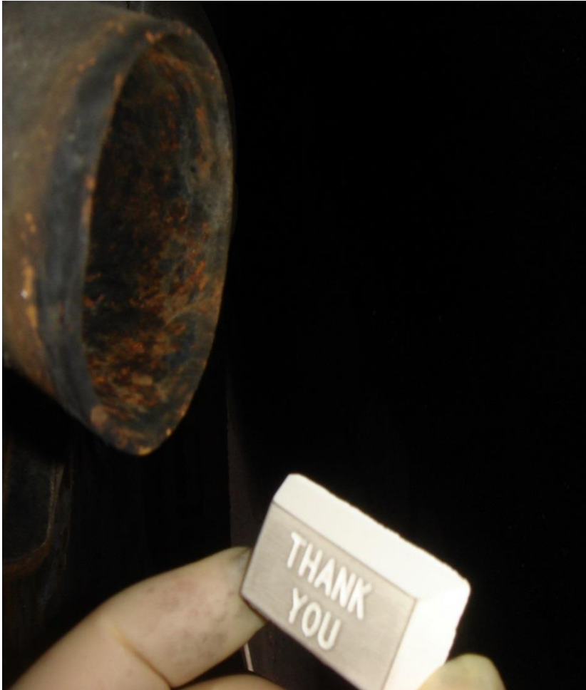
Rubbed with contaminants from automobile exhaust pipe
