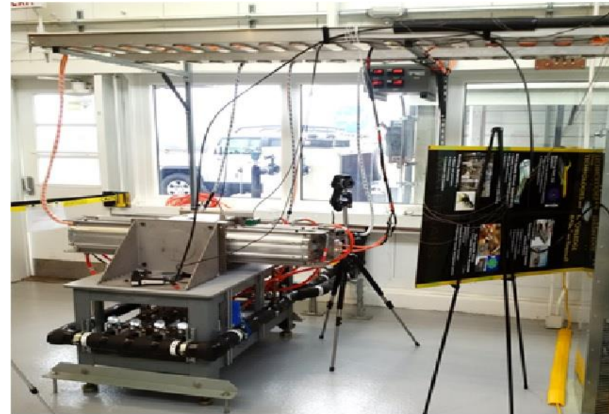
X57 Power Bus Thermal Testing at the NEAT facility
