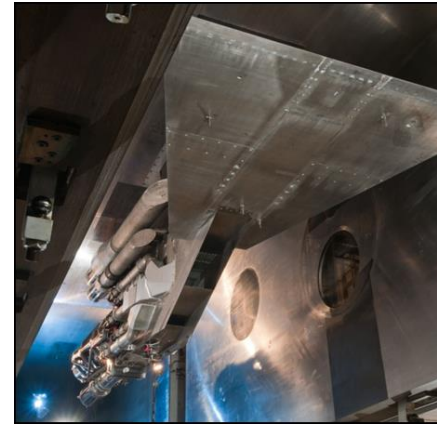
Phase 3C Configuration to simulate turbine engine
