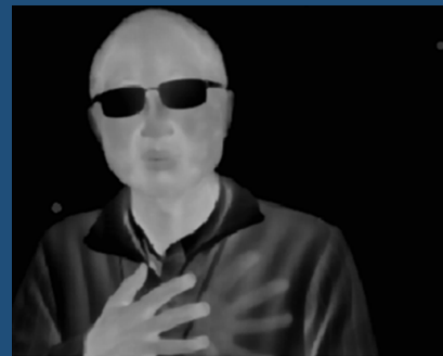
Thermal image taken by a prototype Long Wavelength Infrared (LWIR) Focal Plane Array (FPA) using advanced SLS detector epitaxy materials produced by MBE.
